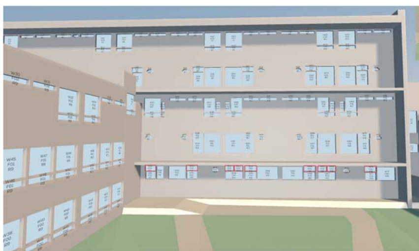
Fig 9: western face of Atlanta Court VSC window failures
